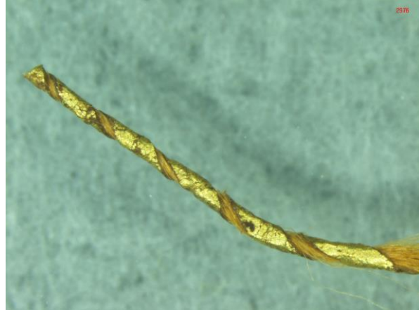
Photo 2. Photo of metal thread sample by stereoscopic microscopy
